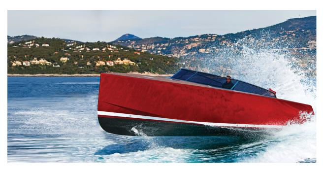
The VanDutch 40 has an axe-shaped bow and clean lines (the cleats are flush-mounted) that make everyone look twice. The cuddy cabin is larger than you would think, and features a V-berth with fill-in cushion, galley and head.
